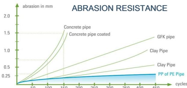
Abrasion curve of various pipe materials according to the Darmstadt procedure
